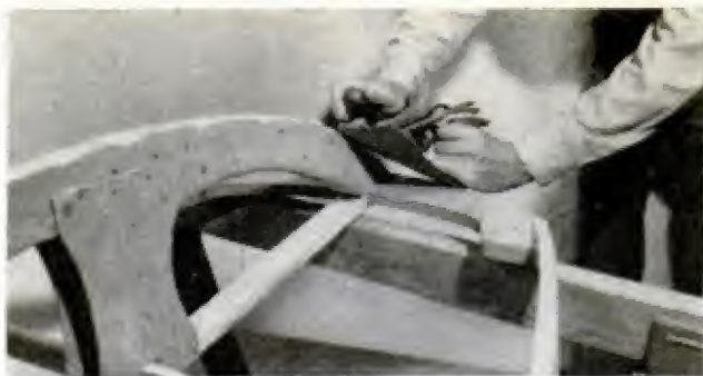
AREAS BETWEEN GROOVES are removed in a smooth, sweeping curve to eliminate any humps or dips
